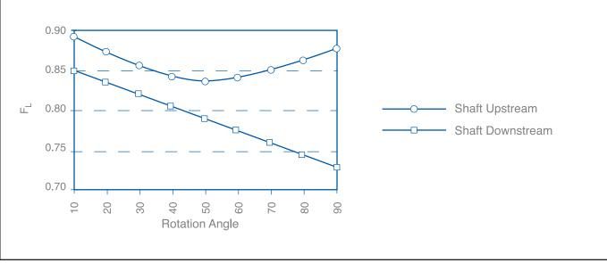
Figure 11: Pressure Recovery Factor, FL: OpEXL Eccentric Plug Rotary Control Valve
