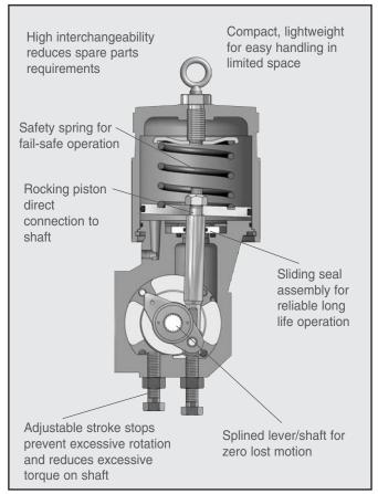
Figure 4: RA Rotary Actuator
