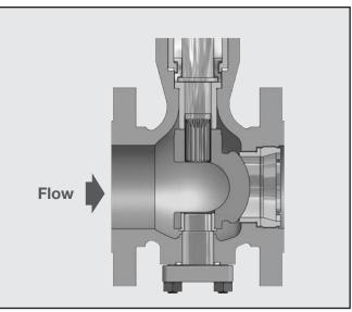
Figure 12: Shaft Downstream
