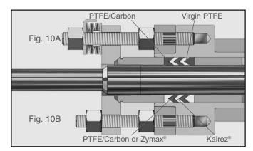
Figure 10A: PT Packing Set Figure 10B: PTG Packing Set
