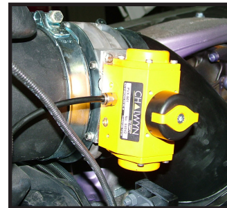
Automatic RPM Overspeed Detection System – Air Pressure Operated, Automatic Reset
