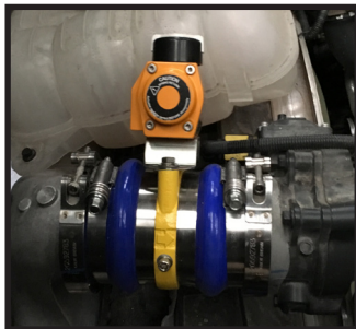
Automatic RPM Overspeed Detection System – Air Pressure Operated, Automatic Reset
