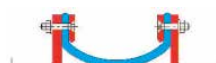
Profile III Installed by means of angle flanges and backing flanges. For negative pressure.
