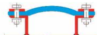
Profile IV Installed by means of parallel flanges and backing flanges. For positive pressure.
