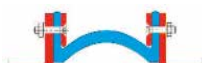
Profile II Installed by means of angle flanges and backing flanges. For positive pressure.
