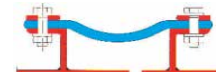
Profile IV Installed by means of parallel flanges and backing flanges. For negative pressure.
